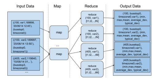
Fig. 3. Diagram of the proposed Map-Reduce implementation
