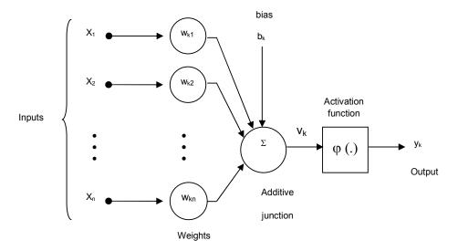
Figure 1. Model of artificial neuron adapted from [1].
